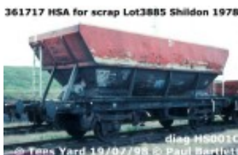
HSA 361717 showing the damage caused by scrap unloading. Tees Yard, 19th July 1998. Paul Bartlett
